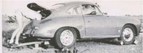
Five-foot plank acts as lever to lift engine into place — all by one person.
